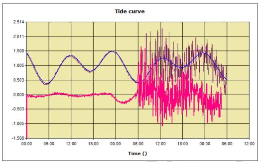
FIGURE 17 – The brown curve is the real signal and the blue curve is the calculated tide corrected with the 2 points procedure while the pink curve is the residual, the difference among the two curves.
