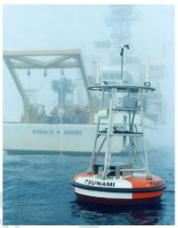
FIGURE 20 – The first operational DART® buoy system design is shown in the photograph on the left (NOAA web site)
