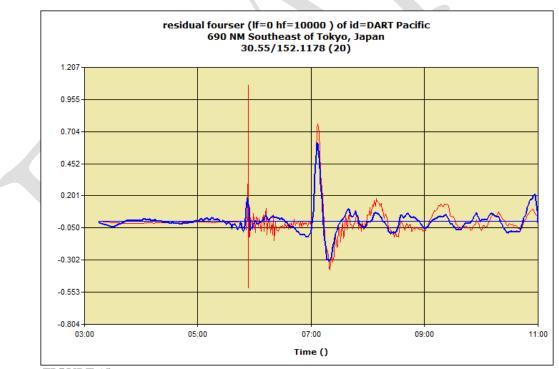
FIGURE 15 - Resulting curve after application of FFT filtering (blue curve) compared with the Moving average with 100 points
