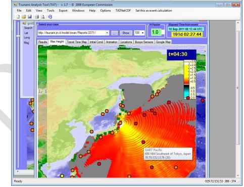
FIGURE 2 – Maximum height with indication of available sea level measurements (circle) and estimated heights on the coasts (rectangles)
