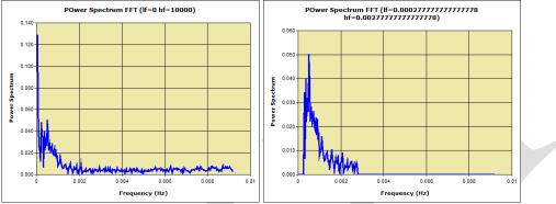
FIGURE 14 – Power spectrof the curve: left without filtering, right filtering high pass filter at 1h (0.00027 Hz) and 6 min (0.0027 Hz) as low pass filtering
