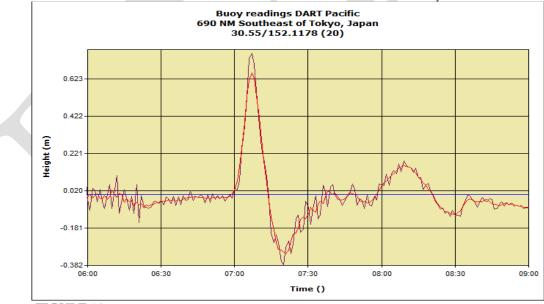
FIGURE 10 – Use of post average averaging procedure (brown curve is with 100 points of Moving average while the in the red curve the residual has been further averaged with 10 points.
